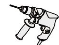
Schlagbohrer (Bohrer: \phi 16\text{mm} )
